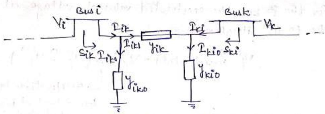
$\pi$ - representation of a line and transformers connected b/w two buses
