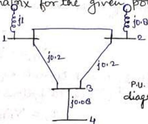
$$Y_{BUS} = \begin{bmatrix} Y_{11} & Y_{12} & Y_{13} & Y_{14} \\ Y_{21} & Y_{22} & Y_{23} & Y_{24} \\ Y_{31} & Y_{32} & Y_{33} & Y_{34} \\ Y_{41} & Y_{42} & Y_{43} & Y_{44} \end{bmatrix}$$
