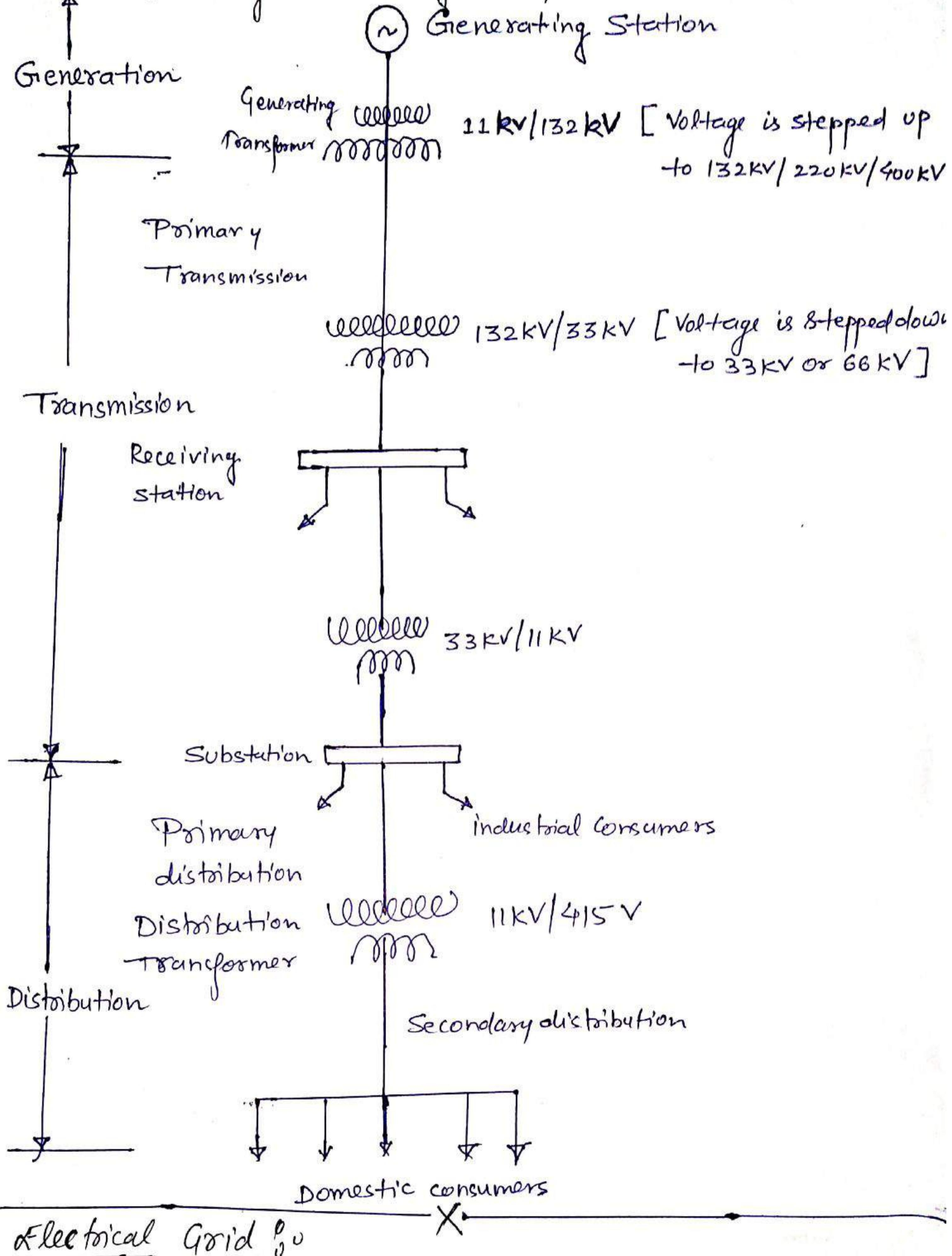
A Grid is an electrical network to deliver power from Generating stations to consumers.
