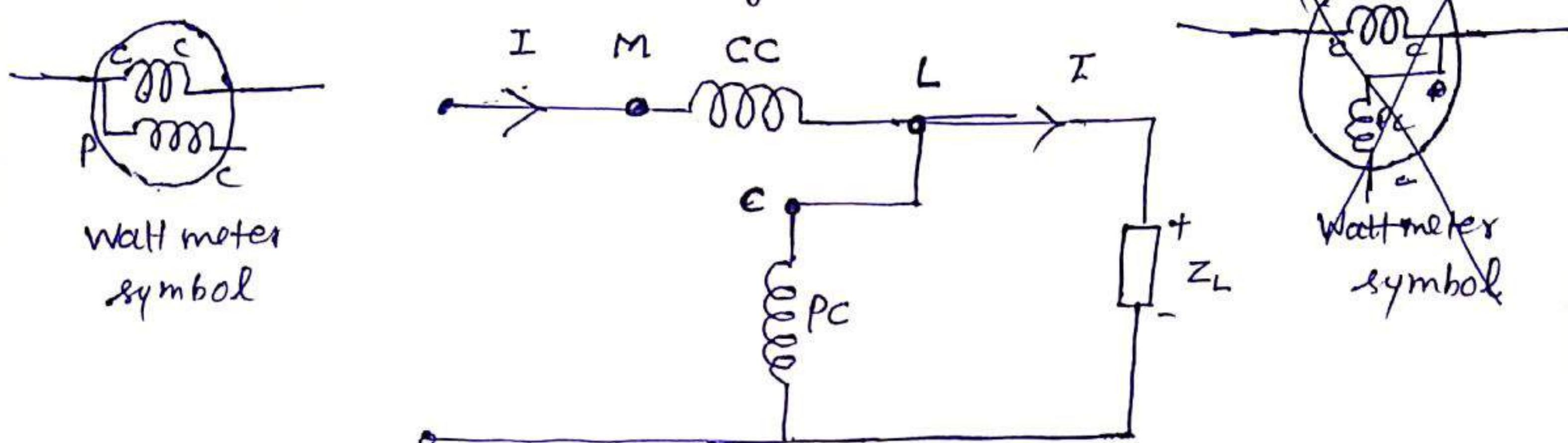
Fig. 1 The wattmeter connected to load
