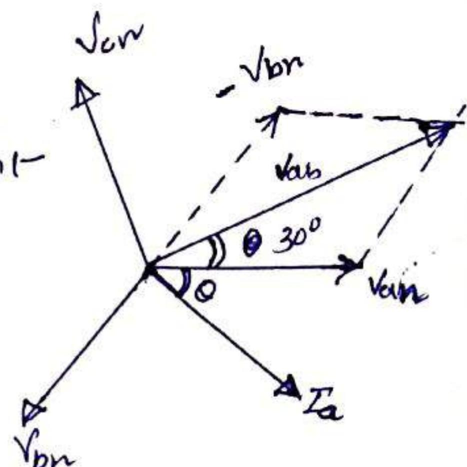
Fig. 3 Phasor diagram for star connection
