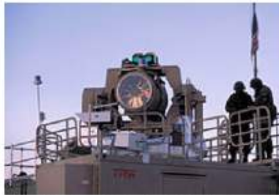
The US-Israeli Tactical High Energy weapon has been used to shoot down rockets and artillery shells.
