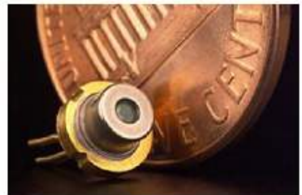
A 5.6 mm 'closed can' commercial laser diode, probably from a CD or DVD player
