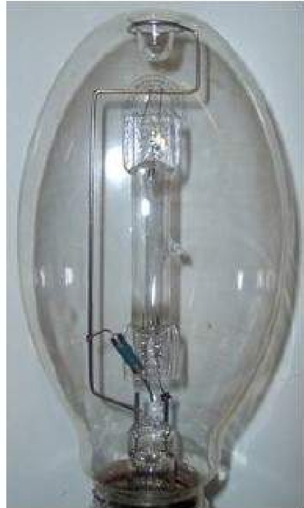
A closeup of a 175-W mercury vapor lamp. The small diagonal cylinder at the bottom of the arc tube is a resistor which supplies current to the starter electrode.
