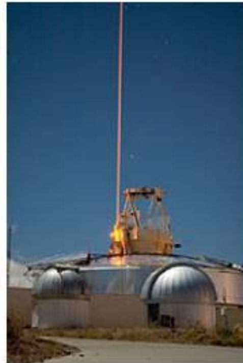
A 50 W FASOR, based on a Nd:YAG laser, used at the Starfire Optical Range.
