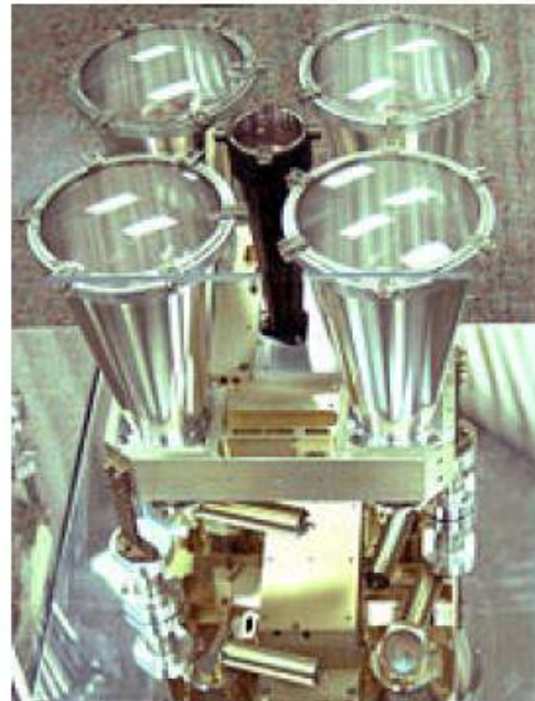
Mercury Laser Altimeter (MLA) of the MESSENGER spacecraft
