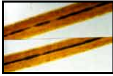
Two matching hairs identified with the comparison microscope
