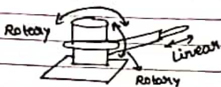
5) SCARA : The term SCARA, is stands for Selective compliant Assembly Robot Arm. The SCARA robot is based on 4-axis design. It is ideal for high speed assembly, fitting, packaging and other material handling applications. SCARA is a world's first direct drive robot.
