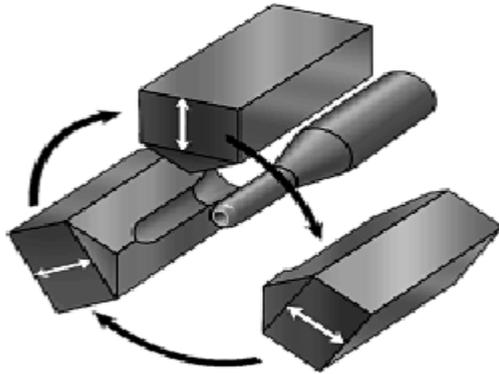
Screwdriver blades and soldering iron tips are typical examples of swaged products. Fig shows these and other products made by swaging.
