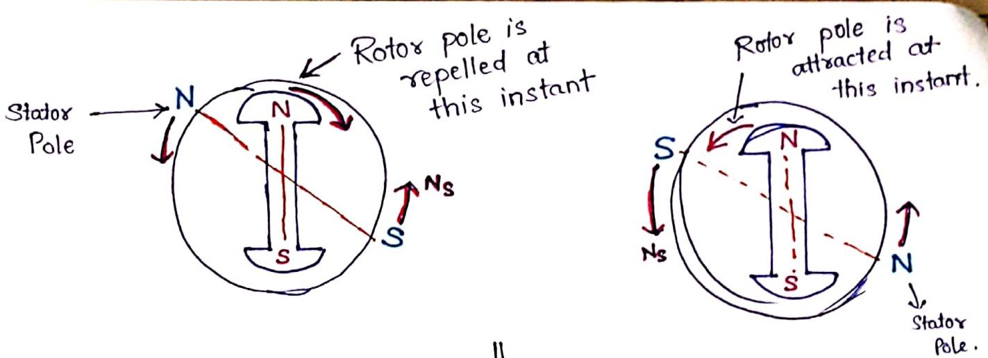
This repulsion and attraction of the rotor pole happens at such a fast pace that the rotor is unable to overcome its inertia and remains stationary.
