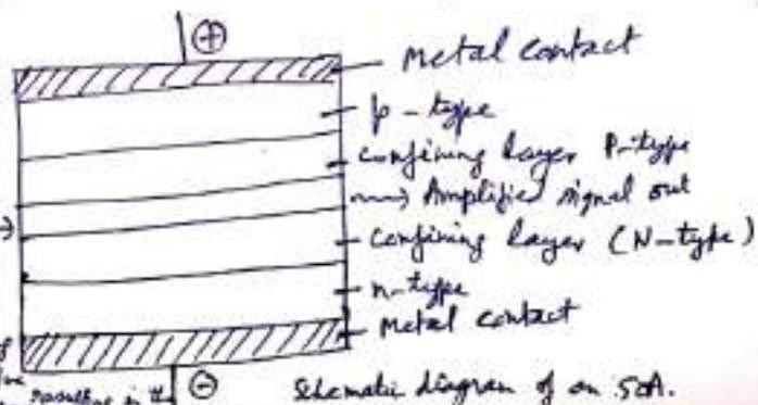
④ Schematic diagram of an SOA.
