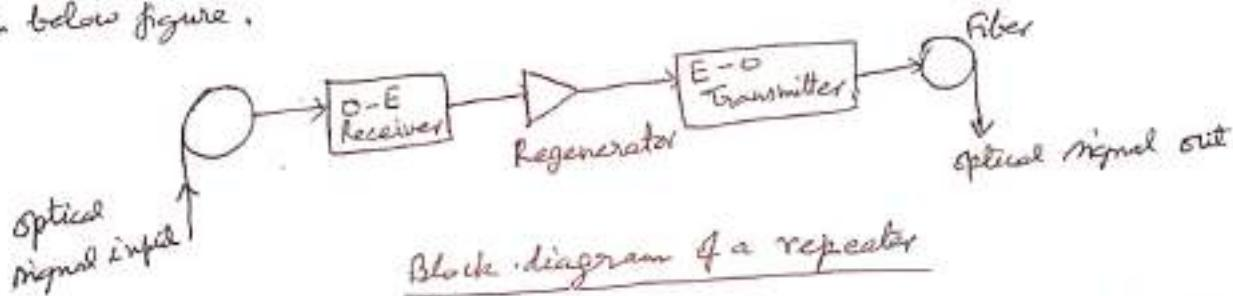
Block diagram of a repeater
