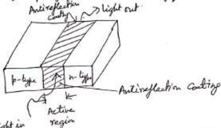
are given an anti-reflection coating to eliminate ripples in the amplifier gain.
