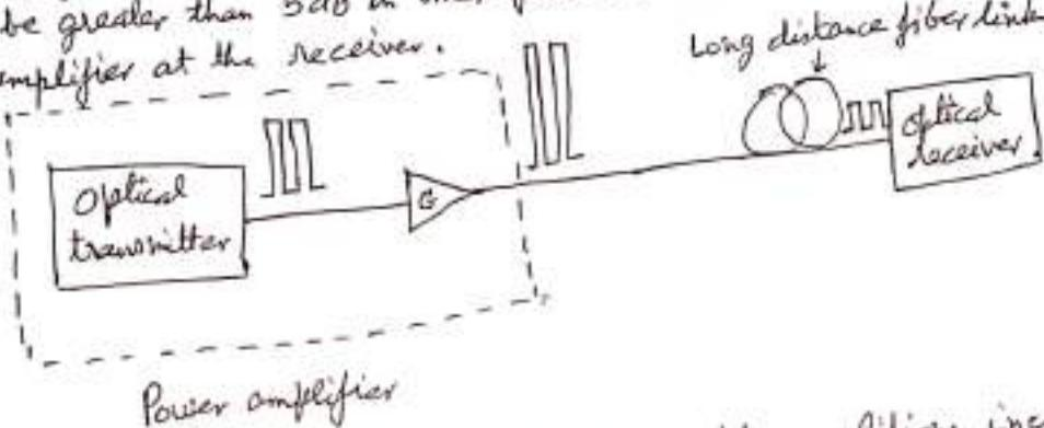
Types of Optical Amplifiers :- All optical fiber amplifiers increase the power level of incident light through stimulated emission or an optical power transfer process. Two main categories of optical amplification are as follows:
