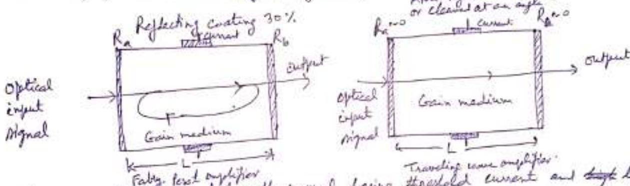
FPA's are normally biased below the normal lasing threshold current and light entering one facet appears amplified at the other facet, together with inherent noise. These devices are very sensitive to fluctuations in bias current, temperature, and signal polarization.
